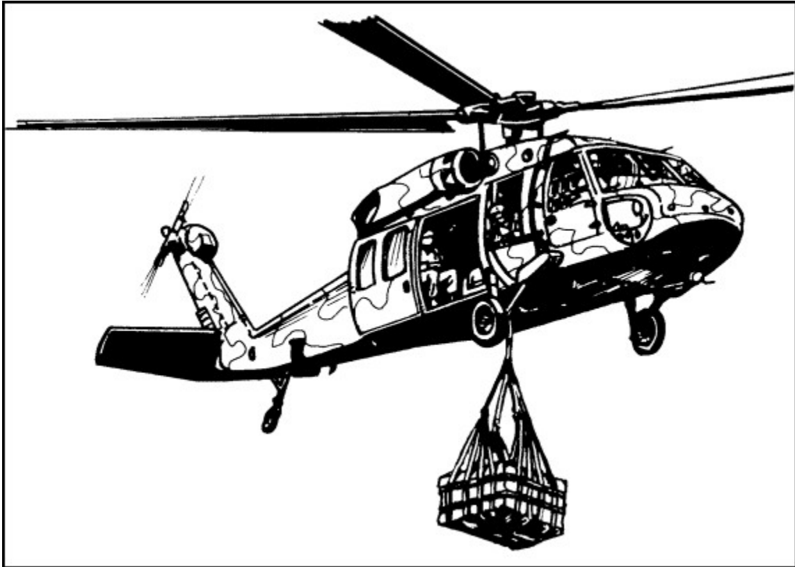
Figure 8-13. Resupply by helicopter.
